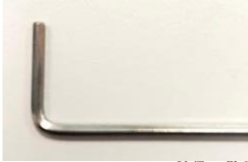
Tighten the M3 set screw by using 1.5mm wrench (not included)
